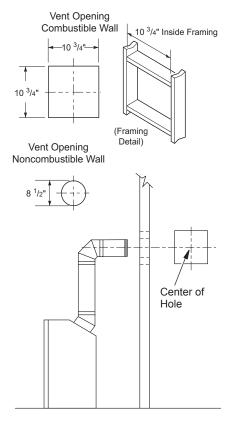
Figure 9 - Vent Opening Requirements
